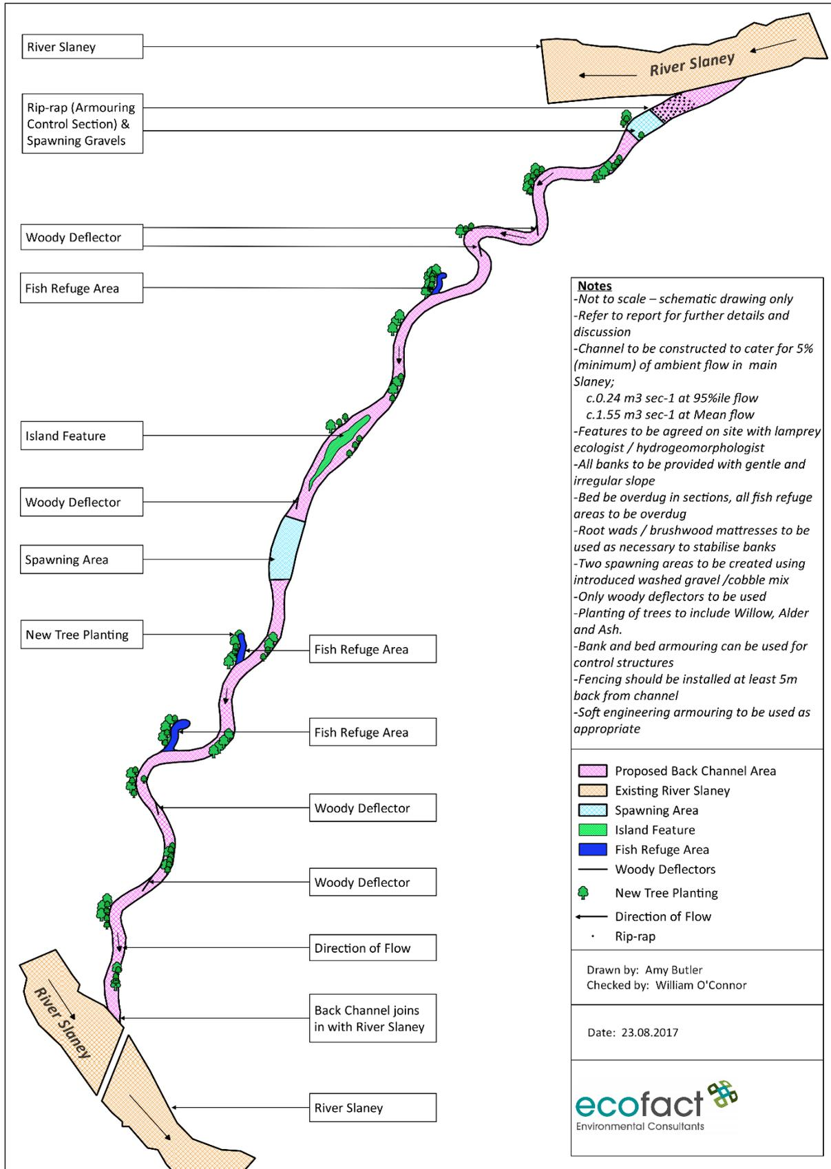
Figure 4 Proposed Back Channel Restoration Schematic Drawing (not to scale).
