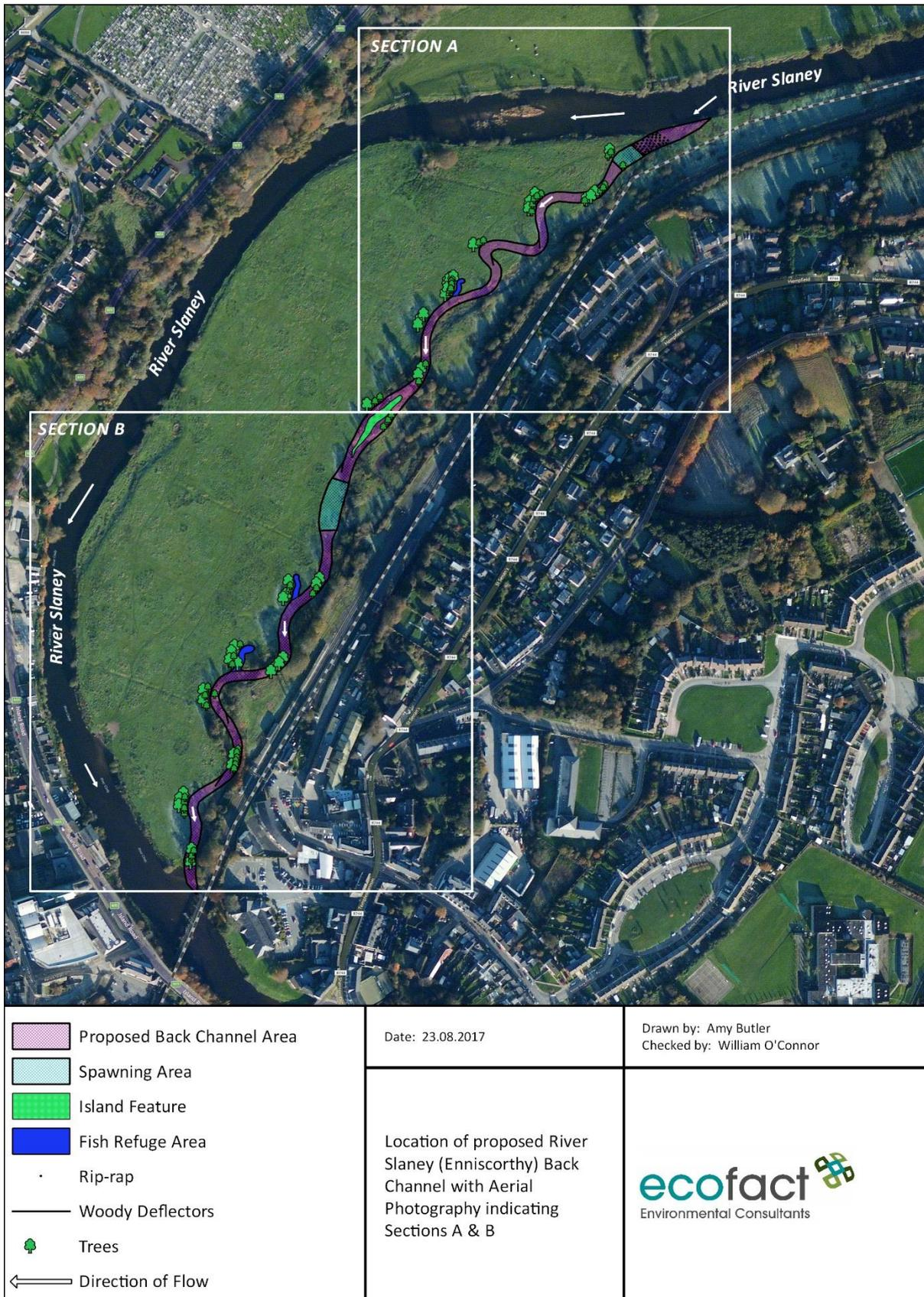
**Figure 1** Location of proposed River Slaney (Enniscorthy) Back Channel with Aerial Photography indicating Sections A & B.
