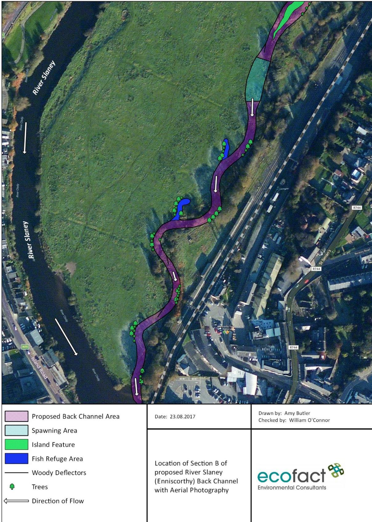
**Figure 3** Location of Section B of proposed River Slaney (Enniscorthy) Back Channel with Aerial Photography.
