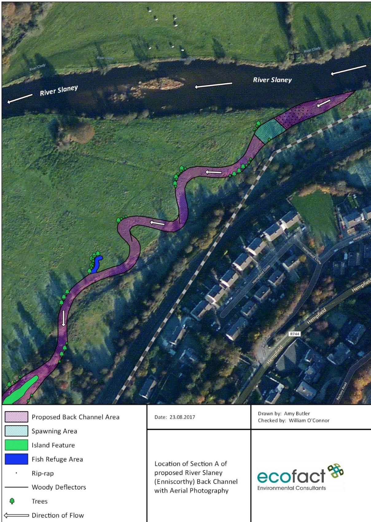
**Figure 2** Location of Section A of proposed River Slaney (Enniscorthy) Back Channel with Aerial Photography.
