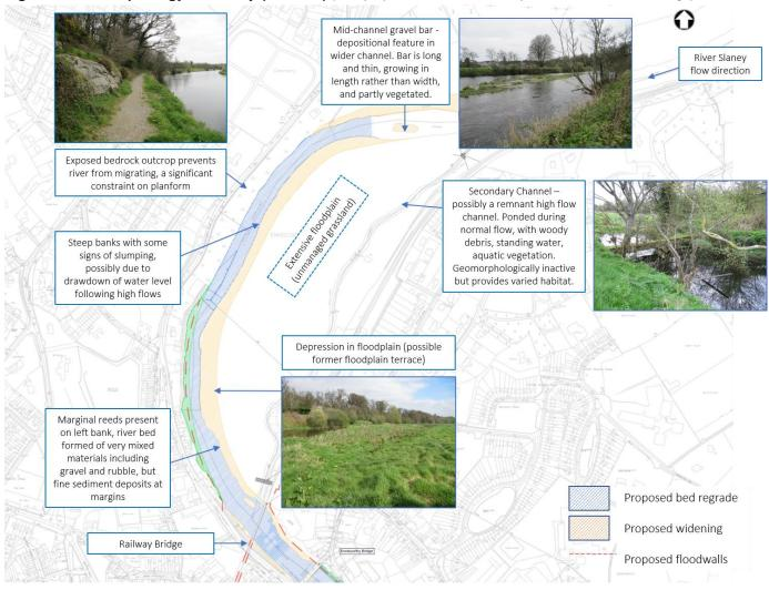
Figure 6: Geomorphology Summary (Reach 1) (note proposed works shown are part of current scheme design)
