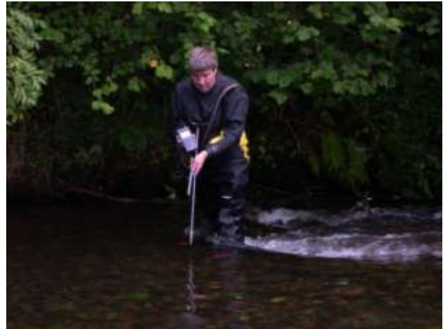
Figure 1 Using a redox meter
